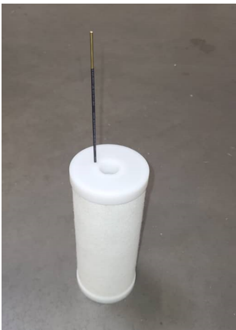
Fig.1 A special electrolysis cartridge in which gold is collected is remelted to produce gold bars.
